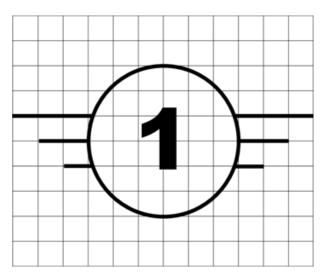
A class C1 UAS bears the following class identification label on the UA:
