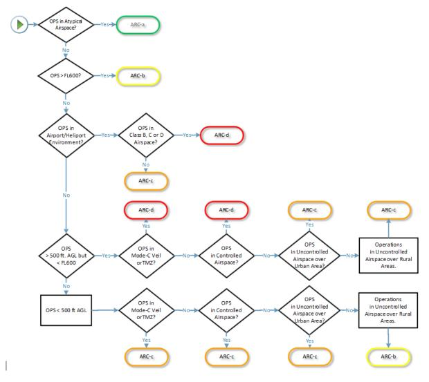
Figure 4 — ARC assignment process
